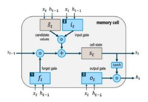
Figure 8: LSTM block architecture
