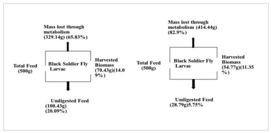
Figure 3: Mass balance across the treatment process, = Mean  $\pm$  standard deviation (n = 3)
